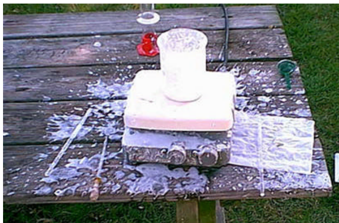
A mixture of barium chloride and potassium bromate explodes from the beaker creating a hazardous situation.
