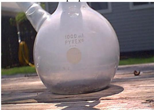
The preparation for boranes is similar to the preparation of silane or of hydrogen sulfide. Acid is slowly dripped over solid magnesium boride ( $MgB_2$ ) resulting in the formation of this spontaneously flammable gas (Note, many boranes are produced, diborane produced is almost instantly hydrolyzed to boric oxide, picture at left shows a milliliter of HCl being dripped onto
