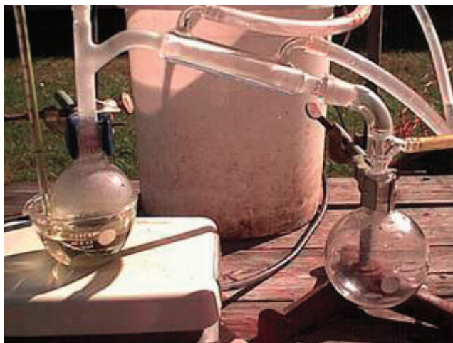
14/20 distilling apparatus, the reaction flask being heated in an oil bath.
